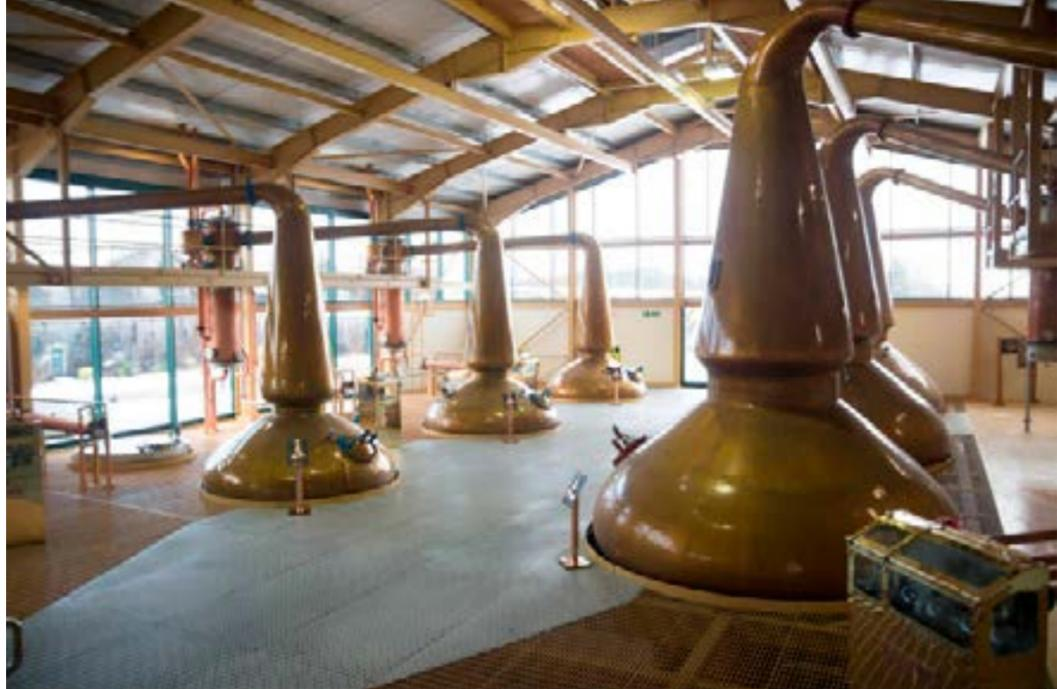
Tall, lantern, or lamp-glass shaped stills, such as these at The Glenlivet, promote a process called reflux, when vapour meets a cooler surface inside the still, turns back into liquid, falls back down the still and is re-distilled. The more reflux there is, the lighter and more complex the spirit will be.
